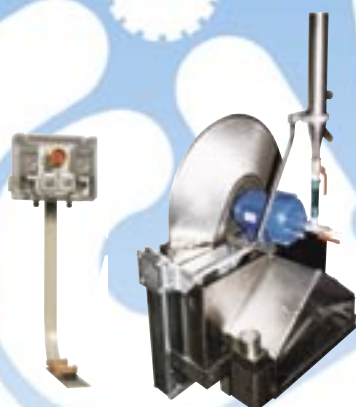
CABINA D. S. JOLLY MOD.F.40 INCLIN. C/MOT. CAVO AZ. INVERTER S.D. TILTING "JOLLY" CABIN, MOD.F.40, W/HOLLOW SHAFT MOTOR DRIVE CONTROLLED BY A FREQ. CONVERTER
