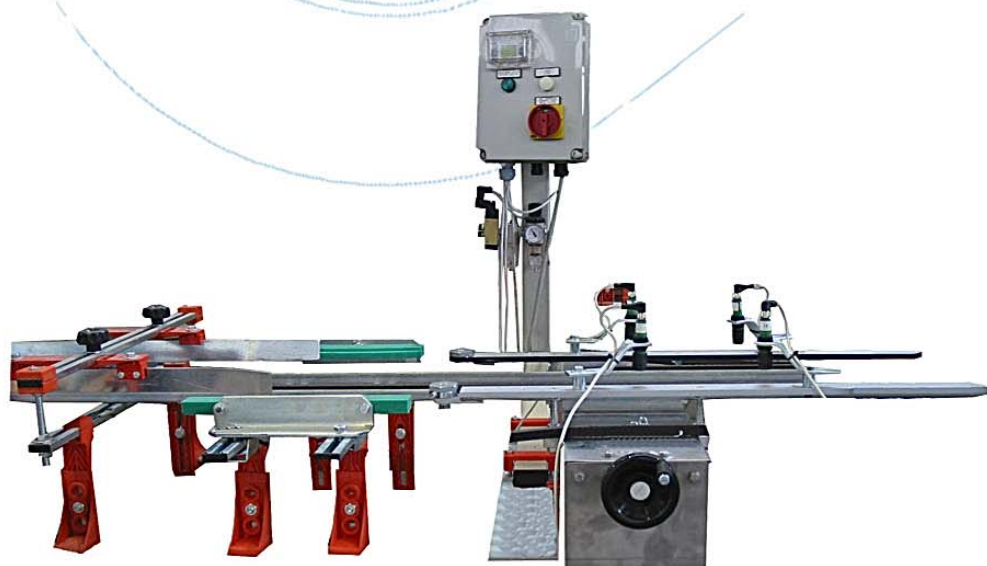
CONTROLLO INTEGRITA' PER PIASTRELLE IN CERAMICA AUTOMATIC CONTROL INTERGITY FOR CERAMIC TILES
