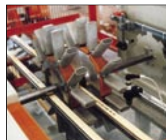
RIBALTINO ELETTRMECCANICO A CROCERA 8 POS. MOD.F.40 ELECTROMECHANICAL TIPPER OF THE CROSS-SHAPED TYPE, 8 POS. MOD.F.30
