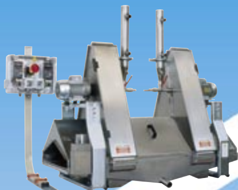
CABINA D. D. CON GRIGLIE MOD.F.40 AZIONATA DA INVERTER D.D. CABIN WITH GRIDS, MOD.F.40, CONTROLLED BY A FREQUENCY CONVERTER
